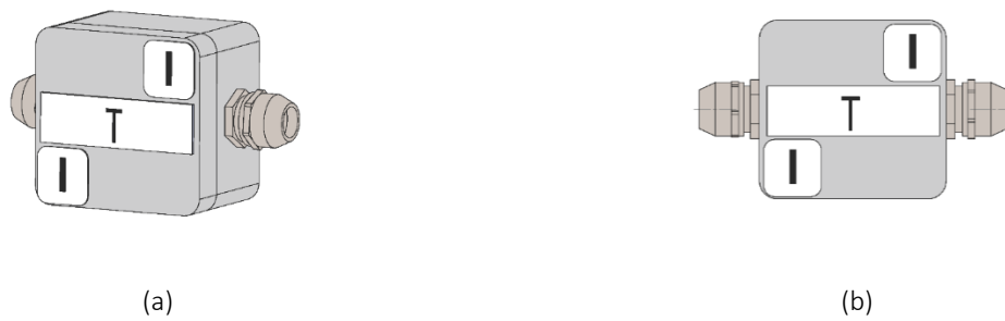
Figure 61. Sealing of Cable Extender Box seen from (a) the front and (b) from the side.
