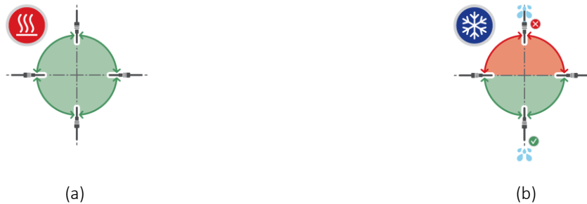
Figure 17. Acceptable orientation of a temperature sensor in (a) a heating and (b) a cooling application.
