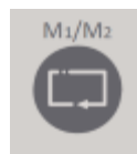
Figure 65. The left push-button shifts between readings/counts of the two flow sensor inputs. In the display, M1 and M2 respectively indicate the currently displayed flow sensor inputs/counters.
