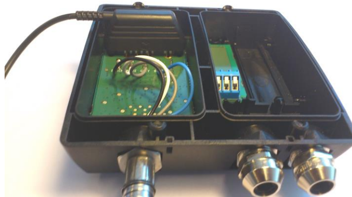
Figure 51. Location of the four-pole connector in ULTRAFLOW® 54 DN150...300.
