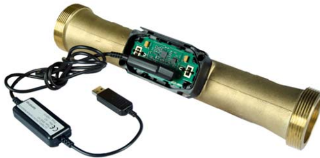
Figure 60. Location of the four-pole connector in ULTRAFLOW® 54 (J).
