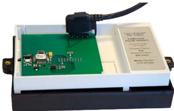
Figure 65. Location of the eight-pole connector in Pulse Divider 66-99-607.
