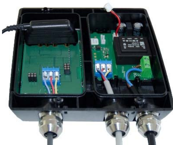
Figure 66. Location of the four-pole connector in Pulse Divider 66-99-907.
