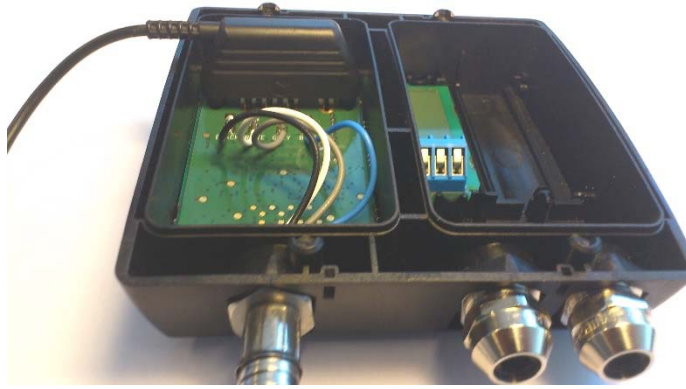
Figure 64. Location of the four-pole connector in ULTRAFLOW® 54 DN150...300.
