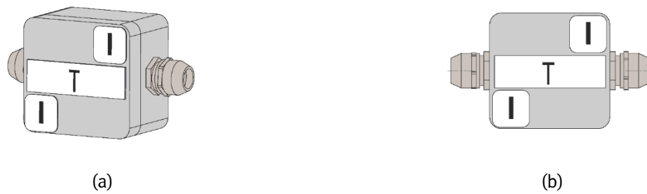
Figure 58. MID-sealing of Cable Extender Box seen from an angle (a) and from the front (b).
