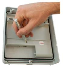
It is recommended to complete the work in the "TEST loop" before starting a reconfiguration via the ""SETUP loop"" or METERTOOL HCW as every reconfiguration is logged in MULTICAL<sup>®</sup> 803 (it is only possible to reconfigure MULTICAL<sup>®</sup> 803 50 times).
