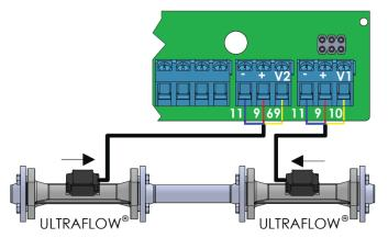
Figure 10 - Installation of 2 ULTRAFLOW<sup>®</sup> for MULTICAL<sup>®</sup> for use for bidirectional flow
