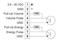
When Pulse Interface type 6699-143 is connected to power supply or battery, the unit is placed on the calculator, and the calculator is in test mode, the following pulses are transmitted:
