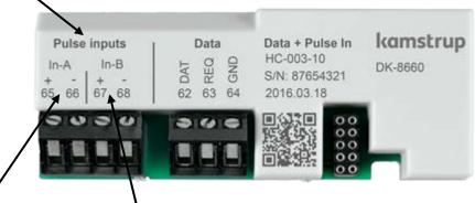
Terminals for In-A and terminals for In-B are marked as well.
