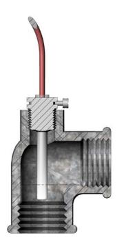
The plastic tube on the sensor cable is placed on level with the sealing screw, which is lightly tightened with your fingers before sealing.
