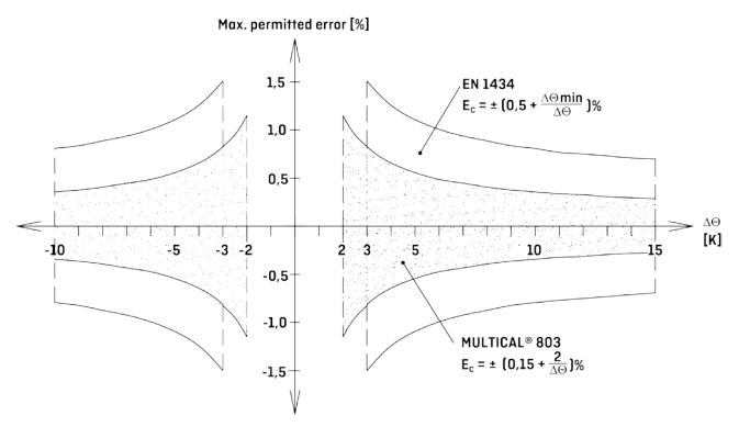
Figure 2: Typical accuracy of MULTICAL® 803 compared to EN 1434.
