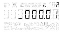
Figure 19 - Setting up positive TL2 in "SETUP loop", the \_ will be flashing when on the sign position but disappears when moving to another decimal.
