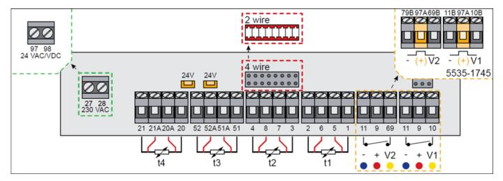
Figure 3: For the use of 2-wire sensor pair, install supplied short-circuit jumper marked in *red*. For the use of internal 24 VDC supply marked in orange, MULTICAL<sup>®</sup> 803 must be delivered with supply type A or C. Additional connection boards for flow sensors with 24 V active/passive pulses (type P) are shown in the upper right corner (6699-045).
