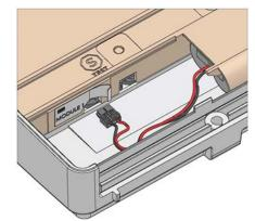
Figure 18 : Socket is moved for backup operation of module slot M1
