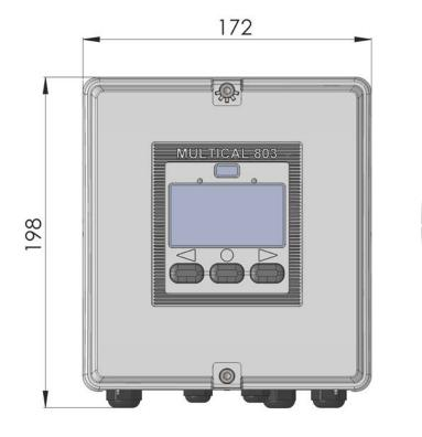
Figure 4: Mechanical measurements of MULTICAL® 803 calculator
