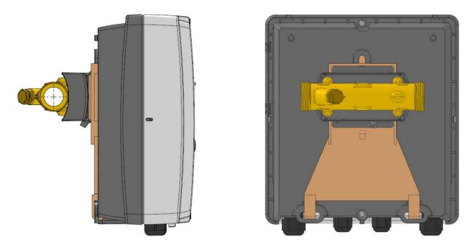
Figure 6: MULTICAL® 803 mounted on ULTRAFLOW® with  $G_{4}^{3}$  x 110 mm threaded connection with bracket 3026-857
