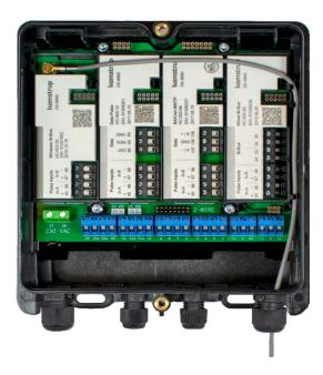
Wireless M-Bus-module with intern antenna
