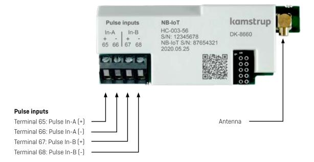
The module is equipped with two pulse inputs, In-A and In-B, to collect and accumulate pulses, e.g. from water and electricity meters.
