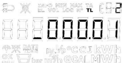
Figure 18 - Setting up positive TL2 in "SETUP loop", the _ will be flashing when on the sign position but disappear when moving to another decimal.
