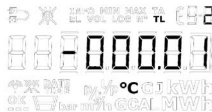
Figure 19 - Setting up negative TL2 in "SETUP loop", the - will be flashing when on the sign position and stay on when moving to another decimal.
