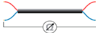
Measurement of cable resistance.
